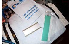
14) The new EL plate (green, it's the backside). The right size is around 8,5 cm x 2 cm ( $\sim$ 3.5 x 0.8 inch); the new plate is larger, no problem! You have to cut it!
