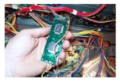
9) This is the Display backside. 3 cables: mid-brown (top), brown and yellow - they'll power your EL-plate from the inverter. CAUTION: The inverter is powering the EL-plate with ~600 Volts, DON'T TOUCH IT when the DSS is powered on!
