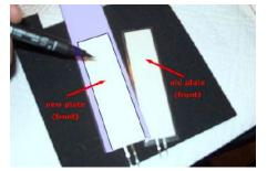
16) Mark with a thin, waterproof felt tip. The lines will be cut too...
