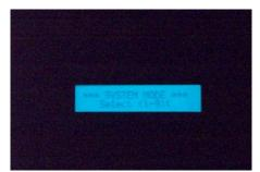
FINAL: This is how it should look like! (After i finally got the zebras matching exactly to the contacts.) Btw: I read about a noizy beep at the Ensoniq ESQ-1 - its the display, if the EL plate does
