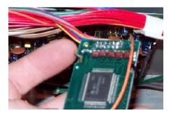
11) This is a bracket (at the finger) fixing the LCD to the board. They're 6 of them. Turn the brackets softly (don't break them!) and turn the display before you lift it!
