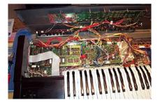
4) Open the DSS board. left side: the Floppy with the cable (I'll add instruction how to replace the Floppy later).
