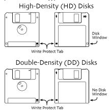
Disks have a sliding write-protection tab so that you can protect your data against accidental erasure. When the write-protection tab covers the protect window, you can store information on the disk. Sliding the tab so that the window is open will protect the disk against being accidentally reformatted or having files deleted. High density disks can be easily identified because they have an additional disk window located on the lower right corner of the disk.
