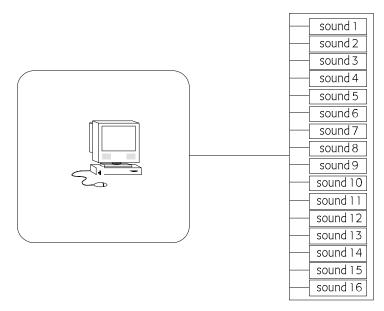
MIDI rigs can also combine both possibilities, with some instruments programmed to respond to one MIDI channel or another, and multi-timbral devices set up to receive up to 16 channels at once.
